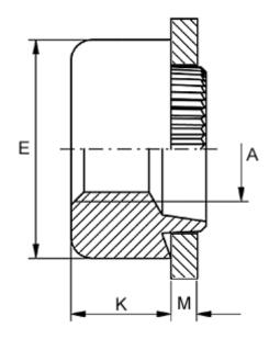
Female thread A = M3,5 Height K = 4.0Outer diameter E = 10.0Plate thickness = 4.7 to 4.9
